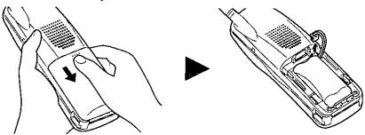
The color cover is held in place by the right and left tabs. Unlock one of the tabs by pressing horizontally (1) and vertically (2), and partially pull down the color cover (3, 4) as shown.
