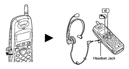
To switch to the speakerphone while using the headset: Press . To return to the headset, press .
